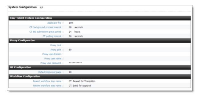
3. To edit a configuration value, click the setting name, which is a link. For example, click **CT polling interval**. The page now displays a description of the configuration parameter and the name of the parameter in the configuration file.
